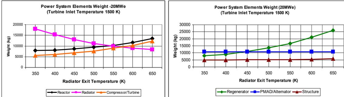
Figure 2. Plot of Weight versus Radiator Exit Temperature for a 20 MWe System
