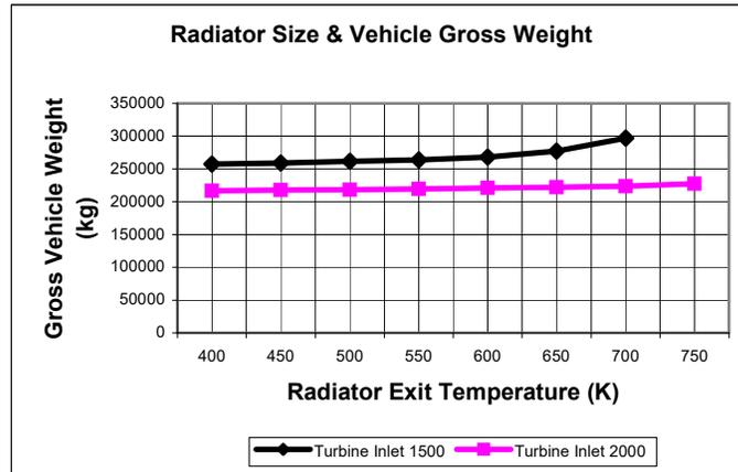
Figure 4 Radiator Size Effect on Vehicle Gross Weight
