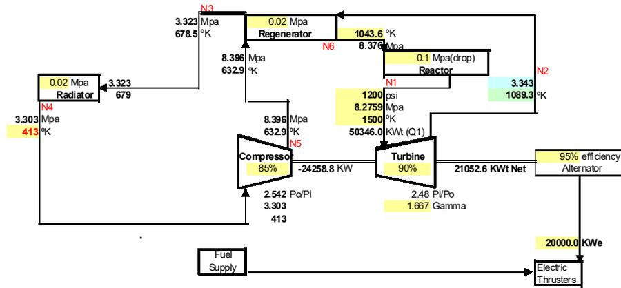
Figure 1. Standard Brayton/ Regenerator Cycle
