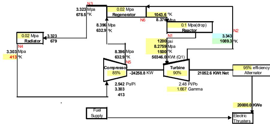
Figure 1. Standard Brayton/ Regenerator Cycle
