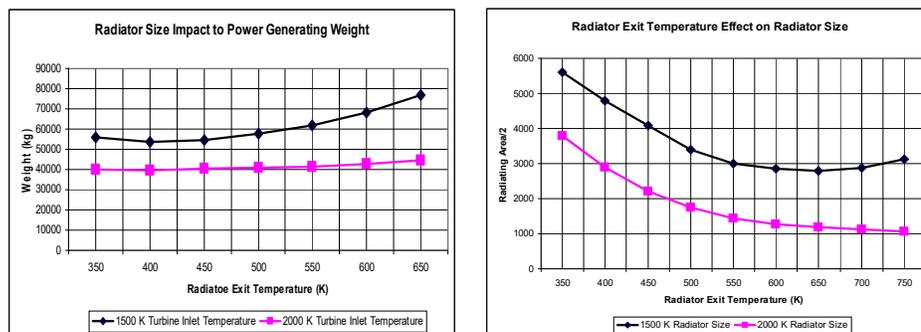
Figure 3. Reduced Radiator Size Effect on Mars Mission Vehicle Total Weight
