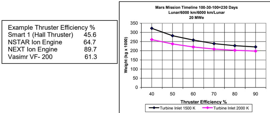
Figure 5. Rocket Nozzle Efficiency Effect on Vehicle System Total Weight
